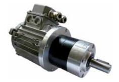
Main advantage of PMS motors against DC motors is the absence of brushes and, as a consequence, lower costs of maintenance; not only, other main features are the constant working torque of PMS motors, working duty which is generating a lower level of noise: 60-70dB compared to 75-85dB of DC motors. Efficiency is also much higher: + 10-15% and, as a consequence, a lower heating and battery consumption.
