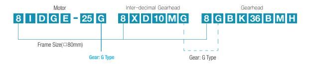
When attaching inter-decimal gearhead, the output shaft type of the motor is always G Type.
