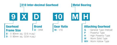
In case of requiring high gear reduction ratio that cannot be generated by single gearhead, please use Inter-decimal gearhead with general gearhead. And please be advised that in this case only revolution speed of output shaft will reduce by 10:1 without increasing of maximum permissible torque.
