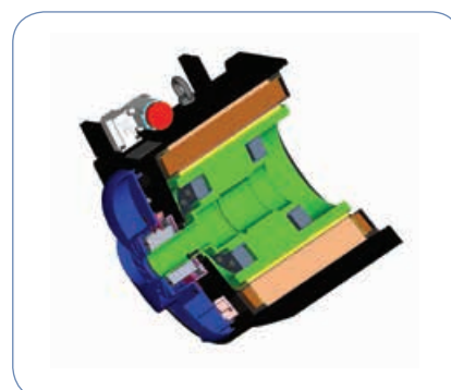
Design of a Cartridge DDR motor (CDDR)
