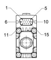
\* Pins 6,9 and 10 must be connected together in user cable connector.
