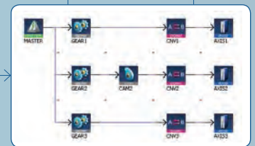
The Pipe Network visualizes a mechanical system in the form of function blocks
