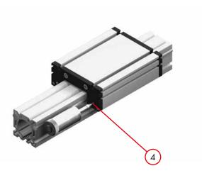
Rods will be greased by the strippers of carriage. There are 2 oil nipples in each wiper end plate (4), where the tanks for the strippers can be filled with an oil gun.
