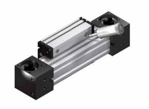
Rollers should be greased each 1.000 working hours or each 6 months with a grease gun. For greaser nipple look at the eccentric at carriage bottom. Use roller grease.
