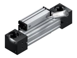
Rollers should be greased each 1.000 working hours or each 6 months with a grease gun. For greaser nipple look at the eccentric at carriage bottom.
