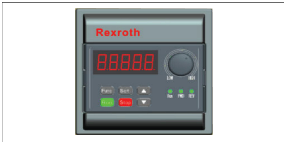
Fig. 15-4: Mount the operating panel (front view)
