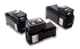
High speed precision microstep drive, controller and stepping motor integrated into one robust package, Ezi-STEP® ALL is unique due to its new control scheme based on a built in high performance DSP(Digital Signal Processor) and software. The onboard controller eliminates costly support systems and can easily digitally network up to 16 axis together to a host controller or operate stand alone.
