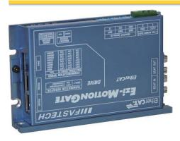
Ezi-Motiongate EtherCAT is Motion Gateway Device that is designed to link TwinCAT PLC, Omron PLC and Industrial PC using EtherCAT protocol to our product such as Ezi-SERVO Plus R, Ezi-STEP Plus R, Ezi-SERVO Plus R MINI, Ezi-STEP Plus R MINI, Ezi-SERVO ALL through EtherCAT protocol. Ezi-Motiongate EtherCAT can support maximum 16 Axes at the same time.
