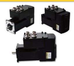
Innovative integrated stepping motor, drive and controller system in one robust package with high resolution of absolute encoder (single turn-262,144/rev and multi turn-4, 096/rev) so it enables to know the previous location even power supply of driver shuts off, Basic functions and specifications are same as Ezi-SERVO-ALL,
