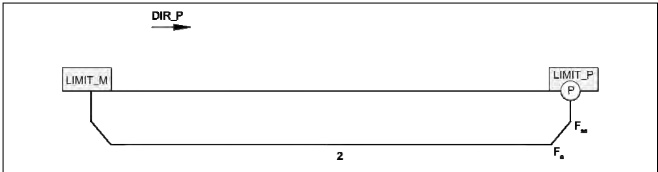
Fig. 28: Start at the limit switch LIMIT_P
