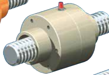
Self-aligning nut PM - Angular compensation up to max. 3° - Bellows can be attached both sides - Uniform Ø on gearbox neck, nut and opposed bearing plate - Grease nipple or connection to central lubrication or lubricator
