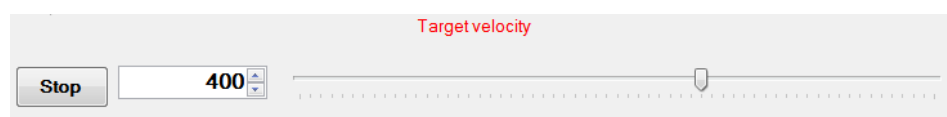
Figure 4.2: Target Velocity track bar is enabled by the RS232 mode when this operating mode has been chosen as Configuration in Programmable Parameters tab.
